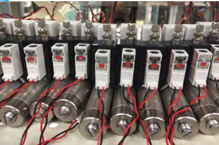
Value-added sub-assembly with custom acrylic manifold
